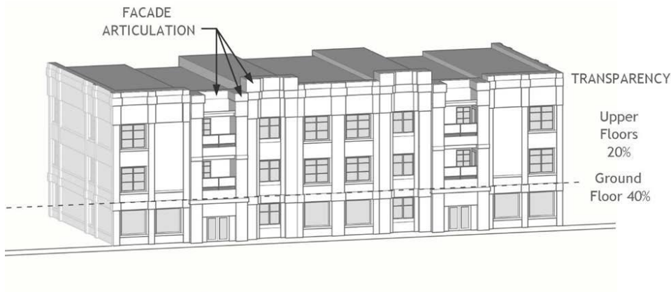
Figure 2-121.F: Façade Articulation, Building Form, and Transparency
